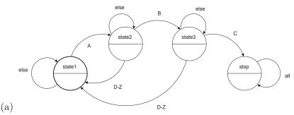
(b) The sequence [A, B, B, C] will cause the machine to enter the stop state, contrary to the specification. The state transition table is fixed below:
