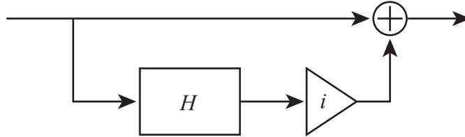
where  $H$  is the Hilbert filter from part (d), and the triangle with an  $i$  scales its input by the imaginary number  $i$ . Note that even if the input is real-valued, the output is likely to be complex-valued. Such a system is called a Hilbert transformer; approximations to it are widely used in digital communication systems.
