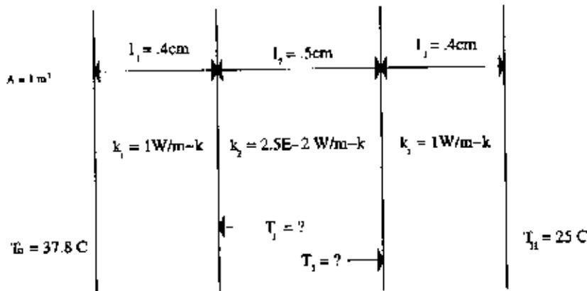
Both panes of glass are identical, with thermal conductivity  $k_1$  and width  $l_1$ . I'm calling the thermal conductivity of the air  $k_2$  and the distance between the panes  $l_2$ , the temperatures on the two inside faces of the window panes  $T_1$  and  $T_2$ , the outside temperature  $T_o$ , and the house temperature  $T_H$  (see diagram).
