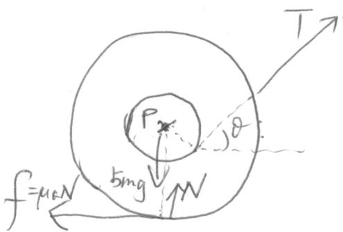
$$\begin{cases} \Sigma F_x = T \cos \theta - \mu_k N = 0 & \text{--- (1)} \\ \Sigma F_y = T \sin \theta - 5mg + N = 0 & \text{--- (2)} \\ \Sigma \tau = \mu_k N R_0 - T R_1 = I \alpha = 0 & \text{--- (3)} \end{cases}$$
