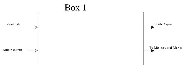
The datapath needs minor changes. Basically, ALU needs to be replaced by GALU1. The Greater1 signal is used to select between \$s1 and \$s2 (so a mux is needed), and another control signal NEWC1 is used to choose between this output and the GALU data output (another mux is needed). In total 1 GALU and 2 mux needed
