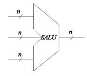
One example of a new MIPS instruction that uses the SALU would be add3 rd, rs, rt, ra ; Reg[rd] = Reg[rs] + Reg[rt] + Reg[ra]
