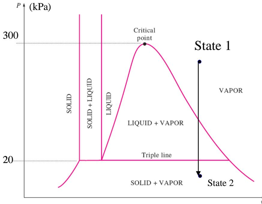
A *rigid* tank contains a pure substance at State 1 as sketched in the above  $(P, v)$  diagram. The pressure at State 1 is 285 kPa. Now heat is escaped from the tank and the pressure inside the tank decreases accordingly. At State 2 after reaching equilibrium, the pressure is 10 kPa. Sketch the process on the above  $(P, v)$  diagram and describe the phase at State 2.
