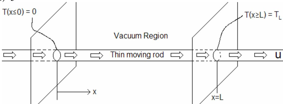
At steady state, a thin solid rod with no radial temperature variation ( $T \neq T(r)$ ) moves at constant velocity  $u$  in the  $x$ -direction. The rod passes through a section of vacuum occupying  $0 \leq x \leq L$ . Outside this vacuum section, for  $x \leq 0$  the temperature of the rod is maintained at  $T=0$ , and for  $x \geq L$  the temperature of the rod is maintained at  $T_L$ . Neglecting radiation in the vacuum section, find the temperature of the rod at  $x=L/2$ .
