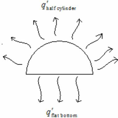
$$q'_{\text{total out}} = q'_{\text{half cylinder}} + q'_{\text{flat bottom}} = h_{\text{cylinder}} \pi R (T_{\text{surf}} - T_{\text{air}}) + h_{\text{plate}} 2R (T_{\text{surf}} - T_{\text{air}})$$
