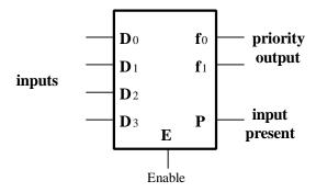
(a) Show a **truth-table** for the priority encoder, in terms of  $D_0$  to  $D_3$  only, and derive the **logic equations** for  $f_0$  and  $f_1$ . Express the logic equations using a **minimum number of literals**.
