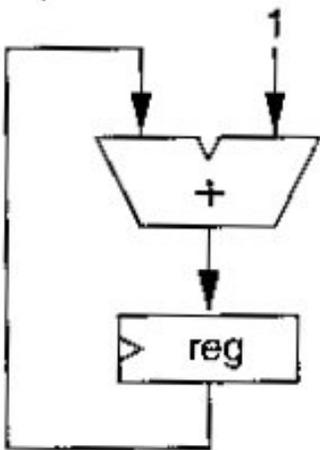
For the circuit shown, assume that the register setup time requirement is 1 ns and the clk to Q delay for the register is 1ns. What is the maximum delay possible through the adder and still guarantee correct operation at 100MHZ?
