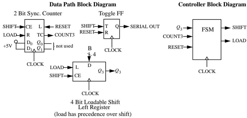
**[10 pts.] b)** Complete the state diagram for a Mealey FSM which will generate the proper control signals for the timing diagram above and proper control of the transmitter. All transitions should be labelled explicitly in the format  $Q_3$  COUNT3/SHIFT LOAD. Use "X" for "don't care".
