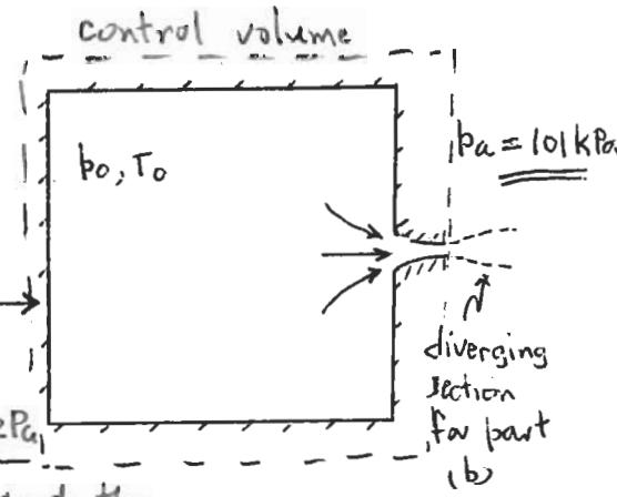
Because  $p_a = 101 \text{ kPa} < b_*$ , the flow is choked and the momentum flow out of the C.V. shown is  $b_* V_*^2 A$ ,  $A$  is exit area. CONCLUSION (+10)
