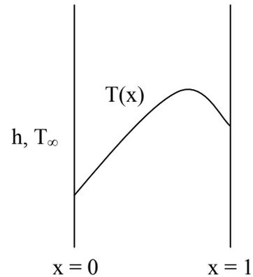
Use temperature distribution to find  $T(x = 0) = 410$  K, thus heat transfer is to the left. At the left boundary the heat rate balance is:
