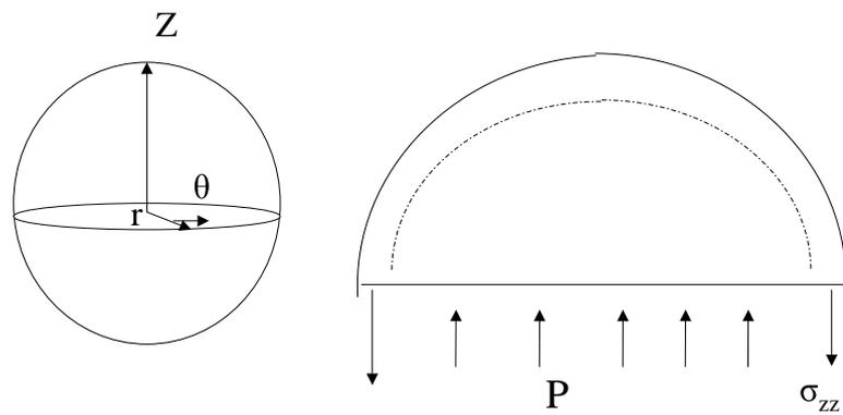
The stresses in the spherical vessel can be found by establishing equilibrium for a section of the sphere as shown above:
