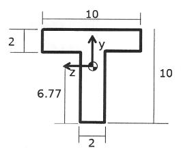
The figure shows the crosssection of a beam. All dimensions are in inches.
