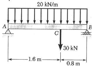
For the beam and loading shown, (a) sketch the shear force and bending moment diagrams (15pts each), and (b) calculate the maximum value of bending moment (5pts).
