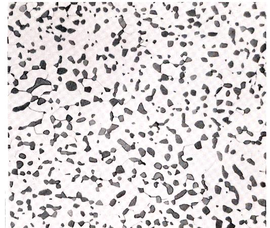
You are entitled to say "**Nonsense!**" At 40 wt%, the microstructure should be single phase  $\beta'$  (phase diagram) but this micrograph clearly shows two phases. Because the alloy was precipitation hardened, the dark phase seen here is the  $\beta'$  phase (lower volume fraction confirmed by tie line) in a matrix of  $\alpha$ . Also from the tie line, the composition is closer to 15 wt% Sn. **The reason for failure must be something else.**
