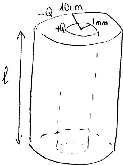
\* This field between  $r = 1\text{mm}$  and  $r = 10\text{cm}$  is  $E = \frac{Q}{2\pi r h \epsilon_0}$  using Gauss's Law with a surface = cylinder of radius  $r$ , length  $h$ .
