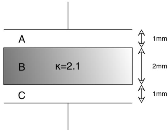
Figure 1: Capacitor with dielectric halfway between plates
