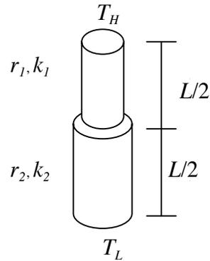
a) Find the heat leak,  $\dot{Q}=dQ/dt$ , from a round wire of length  $L$ . The top half has radius  $r_1$  and thermal conductivity  $k_1$  and the bottom half has radius  $r_2$  and thermal conductivity  $k_2$ . The top end of the wire is connected to a temperature  $T_H$  and the bottom end goes to the experiment at low temperature  $T_L$ .
