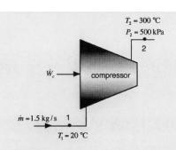
1. Air flows at a steady rate of 1.5 kg/s through a compressor. The inlet temperature at 1 is 20 °C. At the exit location 2, the temperature is 300 °C and the pressure is 500 kPa. The pressure at 1 is unknown, due to an instrumentation failure. The compressor operates adiabatically and has an efficiency of 0.8. In analyzing this system, treat air as an ideal gas with constant specific heats:  $c_p = 1.005 \, \mathrm{kJ/kgK}, \ c_v = 0.780 \, \mathrm{kJ/kgK}$ .
