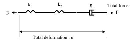
$$F_1=k_1u_1 \\ F_2=k_2u_2 \\ F_3=\eta^*(du_3/dt) \\ F_1=F_2=F_3=F$$
