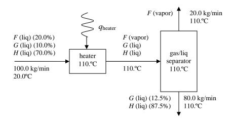
**8.** (20 points) In the scheme shown below, calculate  $q_{\text{heater}}$  in kJ/min.
