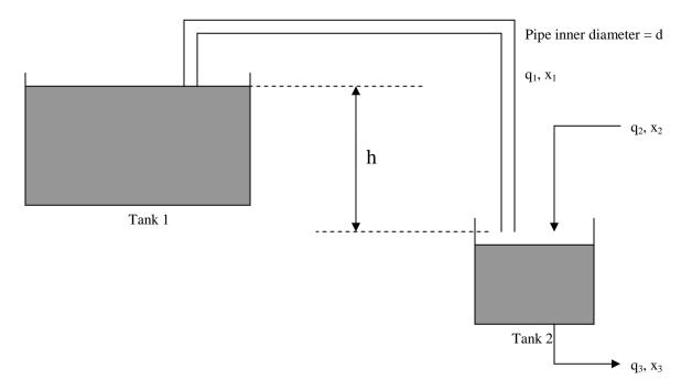
Stream 1 is the undiluted wastewater, stream 2 is the pure water used in the dilution, and stream 3 is the diluted wastewater that goes on for more processing.
